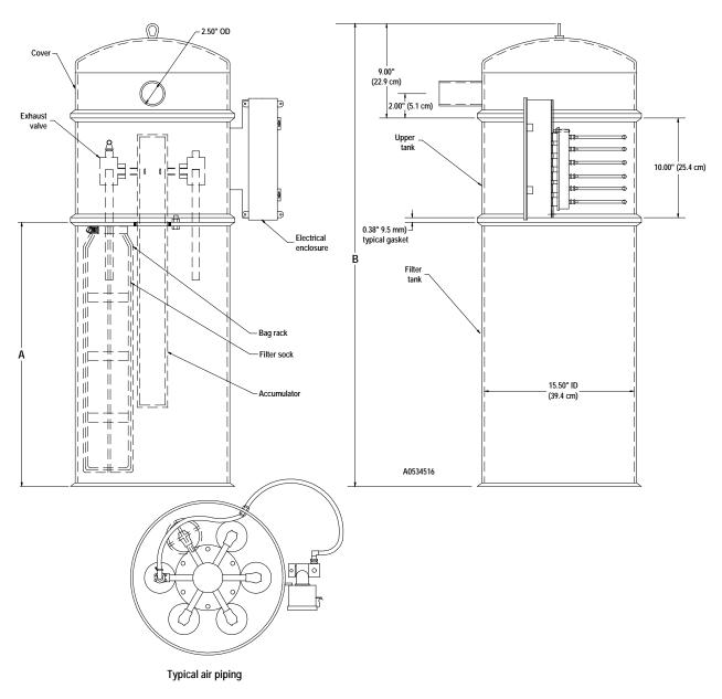
Figure 14: Typical ACA Series Filter Chamber
